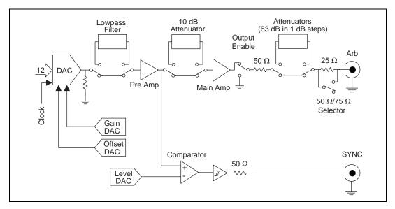
Figure 2-8. Analog Output and SYNC Out Block Diagram
